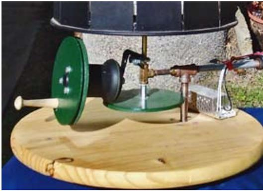
This view shows the concentric axle and drive mechanism for operating the independent floor at the bottom of the aperture or palisade drum.
